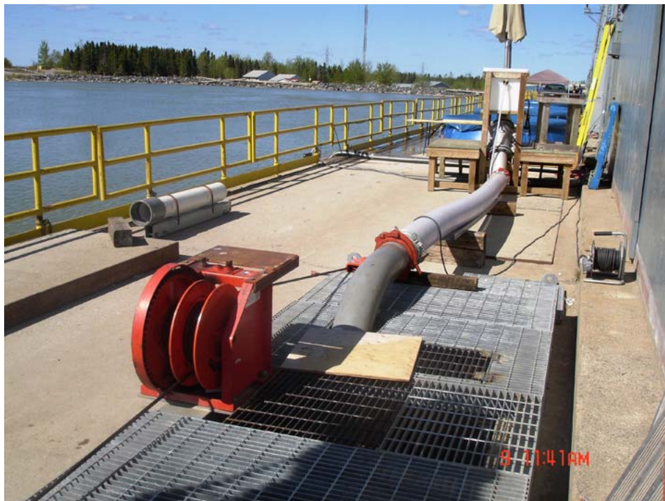
Figure 2-9 Induction apparatus (upper photo) and release pipe (lower photo) for introducing fish into Unit 5 Turbine intake at the Kelsey GS.
