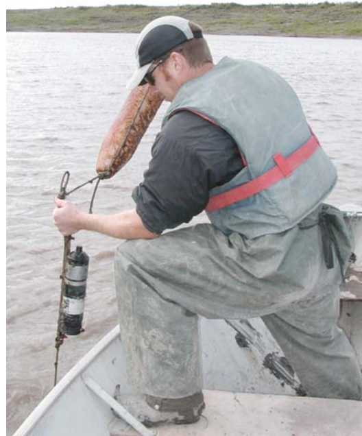
Figure 8. Deployment of a stationary VR-2 receiver, also showing steel cable and float.
