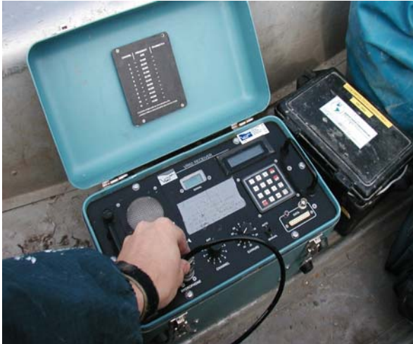
Figure 9. VR-60 acoustic receiver used for manual tracking of fish in June and August.
