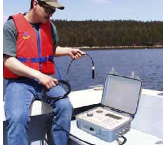
Figure 10. VR-100 acoustic receiver used for manual tracking of fish in October (from http://www.vemco.com ).
