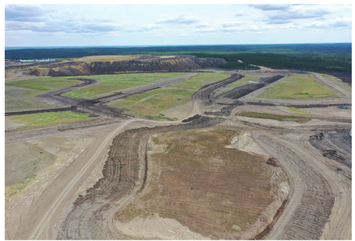
Tailings Management Area (TMA) The clay capping starting to green up with vegetation
