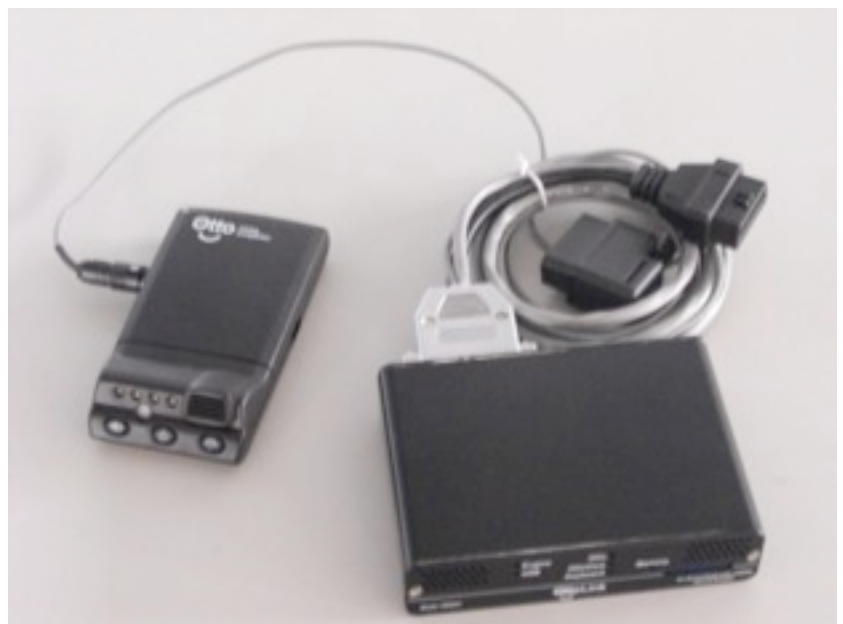
PQL electricity data-logger (left) and Otto Driving Companion logger and Otto-Link CAN-Bus logger (right)
