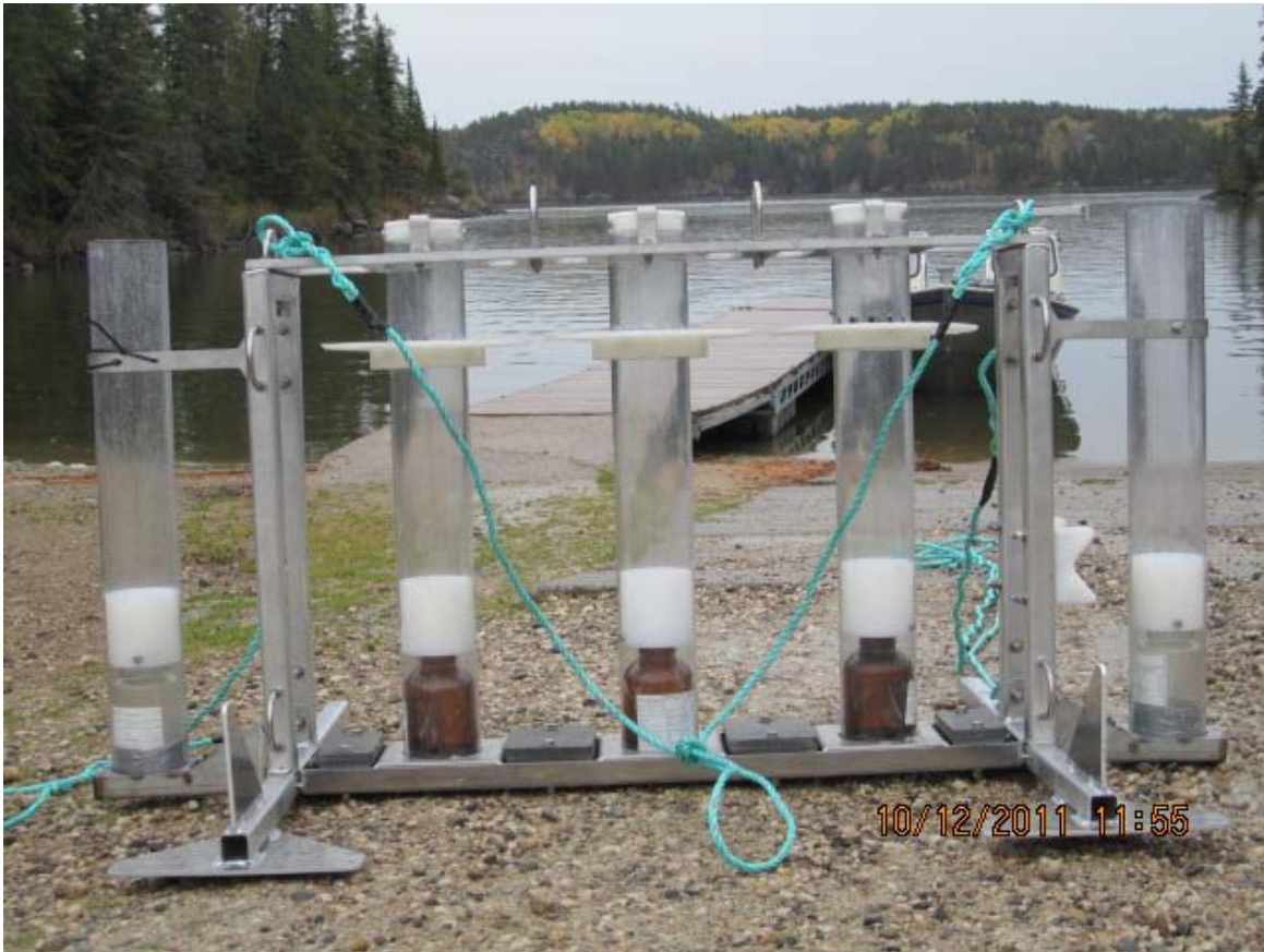
Figure 2-3. Sedimentation monitoring equipment (Sediment traps), Pointe du Bois Spillway Replacement Project.
