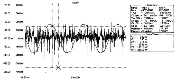
Glenn Wylds Input A(blue wave) is 120 volt receptacle. Input B(red wave) is the high frequency riding on the 120 volt sine wave. This was recorded before the house was filtered. Stetzer meter reading of 200
