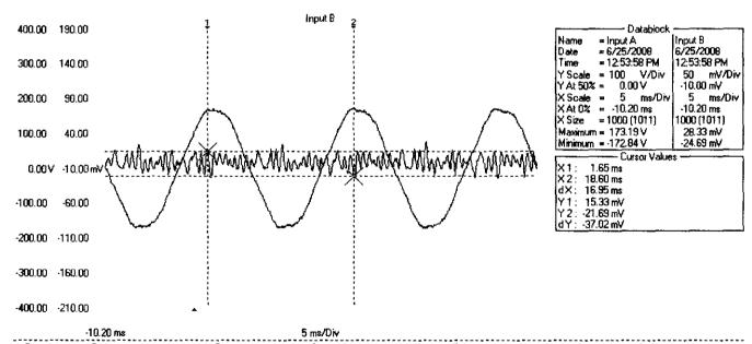
Glenn Wylds Input A(blue wave) is 60 hz 120 volt wave. Input B(red wave) is the high frequency riding on 60 hz wave. House filtered with Stetzer filters and Powermedix Filter at the panel. Graham-Stetzer meter reading 22-27.
