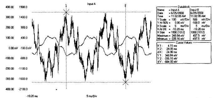
Glenn Wylds Input A(blue wave) is PNEV. Input B(red wave) is sink to floor.
