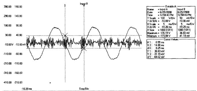
Glenn Wylds Input A(blue wave) is the 60hz 120 volt sine wave. Input B (red wave) is the high frequency riding on the 60 hz wave. The Stetzer filters installed, no powermedix. Graham-Stetzer meter reading of 25-30. Notice this pulsating harmonic wave I am assuming is coming from the windmills.
