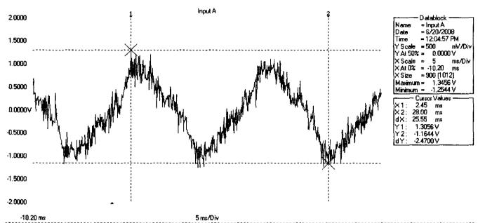
Doug Eadie PNEV windmills on neutral now isolated ground wire in ditch now. High frequency being induced onto Doug's Neutral from 3 phase collection line from windmills ?
