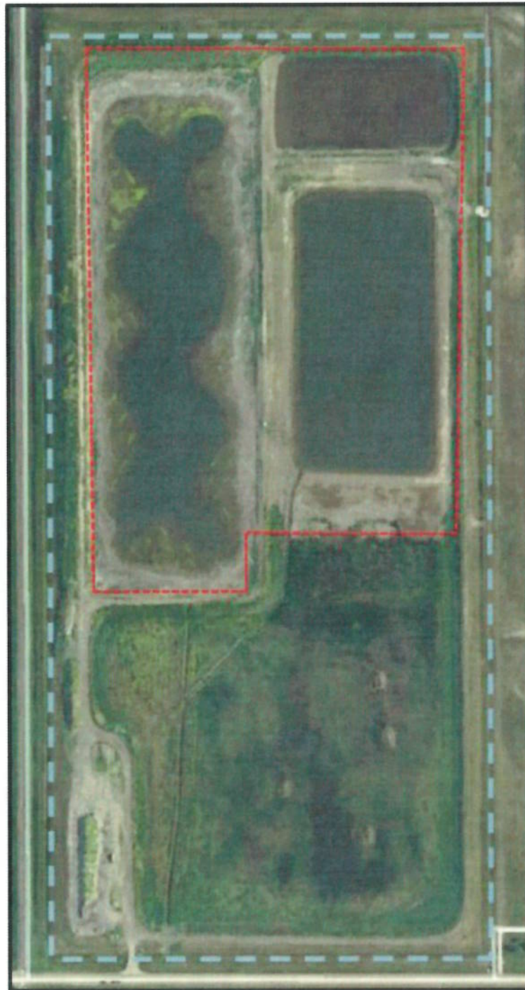
Figure 4. Outer 1.2 m fencing location around perimeter of old lagoon site (light-blue, dashed line) and inner 1.8 m fencing on the inside of the lagoon berms around areas remaining under licence (i.e., control, holding, and wetland cells). Note that the fencing locations shown are approximate and for discussion purposes only. Image courtesy of Google Earth (Imagery date: 2013).
