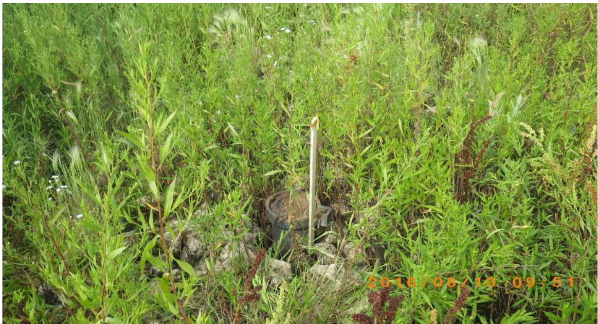
Photo 1: Low level sampling pipe steel protective casing.
