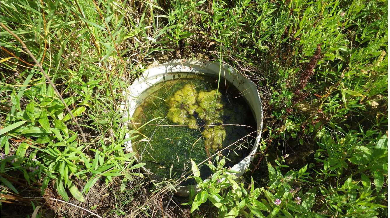
Photo 2: Low level sampling pipe and protective steel casing at 5A1. Cover is missing.
