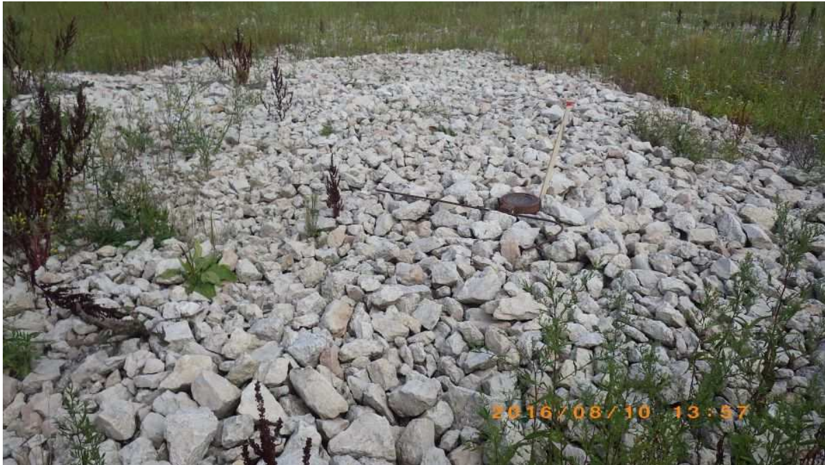
Photo 1: Spring treatment filter site 17A2 and low level sampling pipe.
