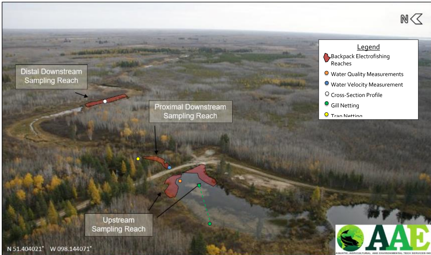
Figure 11. Aerial photograph of Crossing 2 taken on October 9, 2015. Fish sampling reaches indicated in red. Water temperature and turbidity measurements performed at orange point; culvert output flow velocity and turbidity measured at blue point; velocity and substrate profile measured at white point; gill netting performed at green point; trap netting performed at yellow point.
