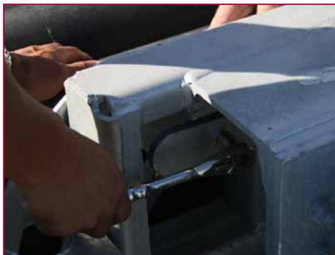
Bolting EAE to Compact Backstop
