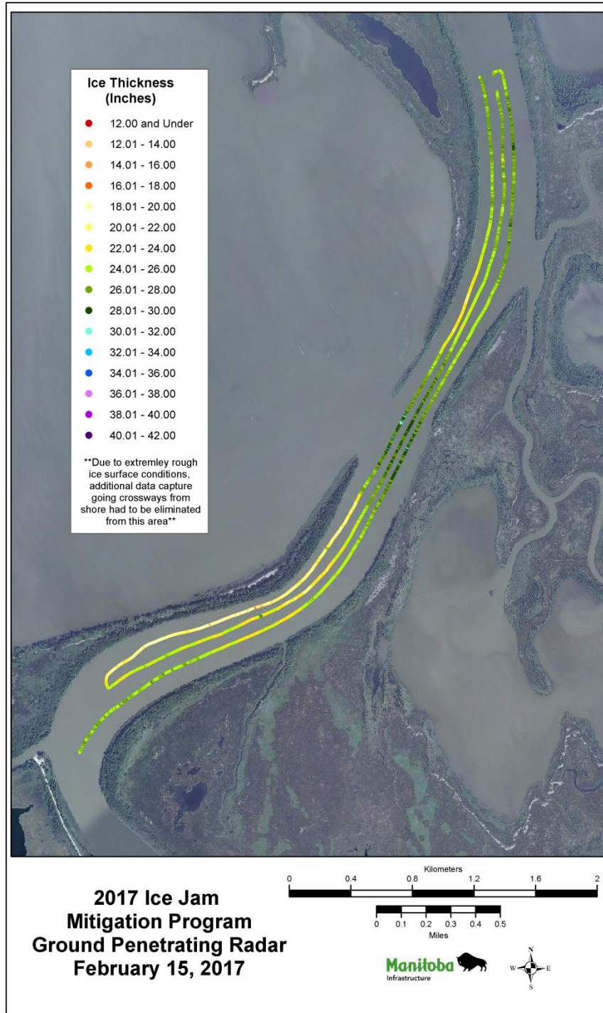
Figure 10 – Ice Thickness Measurements based on Ground Penetrating Radar, Netley North
