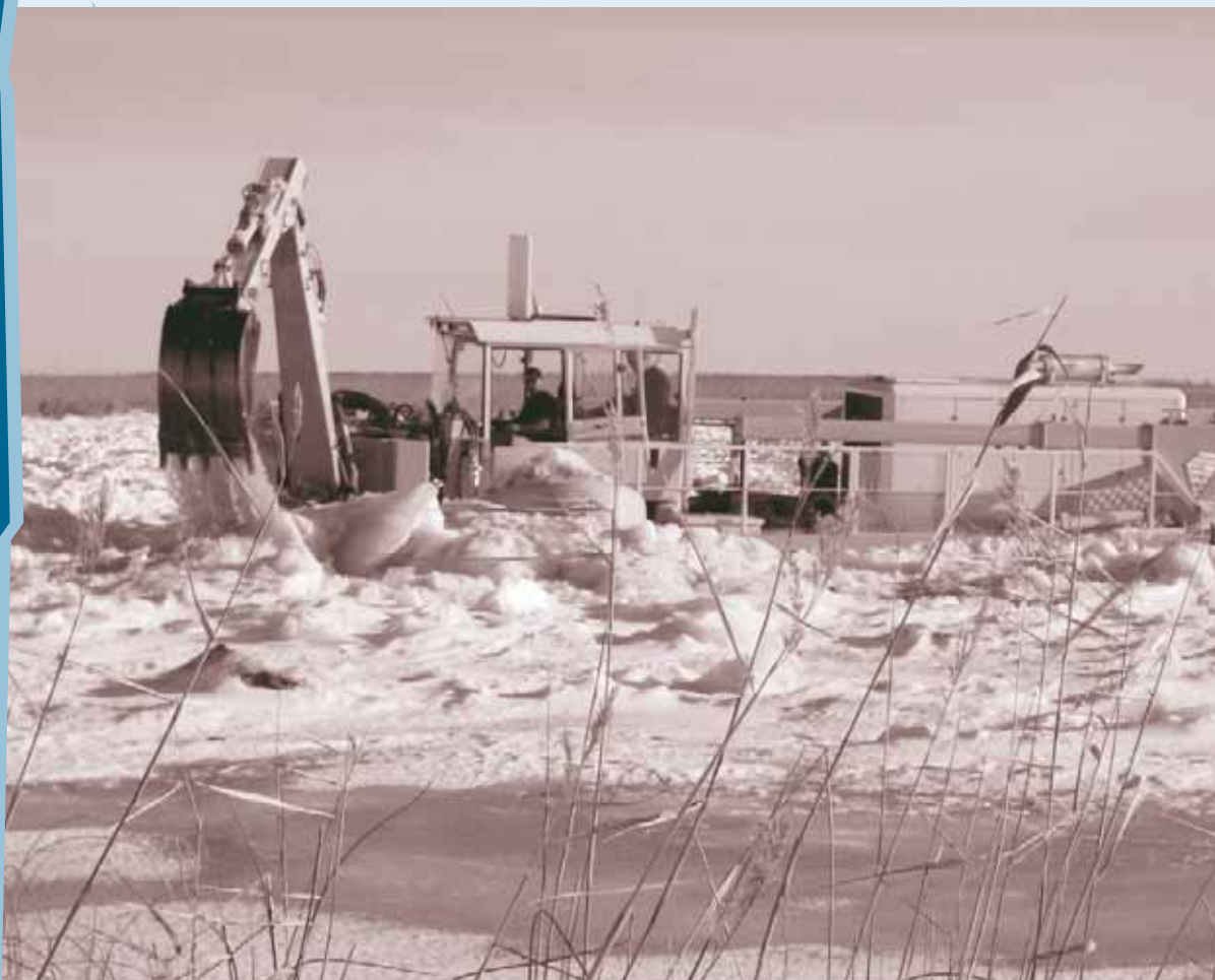
The Canadian-made Amphibex excavator breaks up ice jams near Waterhen in November 2006 to help reduce flooding.
