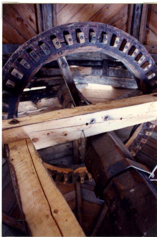
This view of the wooden sprocket of the Hykawy Mill demonstrates that much of the mill has been reconstructed. (H.R.B. photo, 1991)
