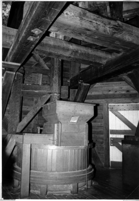
The second, working set of millstones is enclosed within a wooden drum and is used to mill flour which can be purchased at the museum's visitor centre. (H.R.B. photo 1991)
