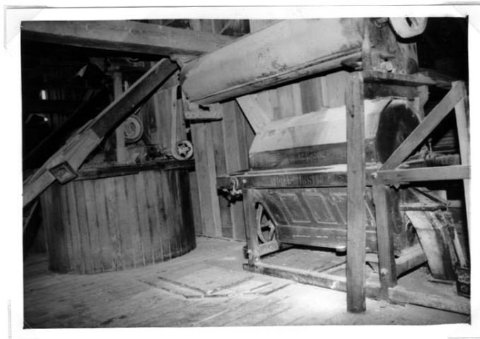
Interior view of the Barkman Mill, Steinbach showing a bran duster. (H.R.B. photo, 1991)
