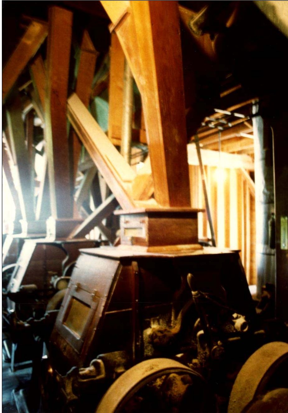
Harrison Bros. Mill, Holmfield. Interior view showing the flour rolls. (HRB photo, 1991)
