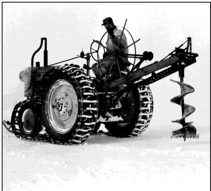
Tractor with ice auger. The use of tractors with motorized ice augers eliminated the need for laboriously chopping holes in the ice. (Source: Water Stewardship, Fisheries Branch Collection, C10571.)
